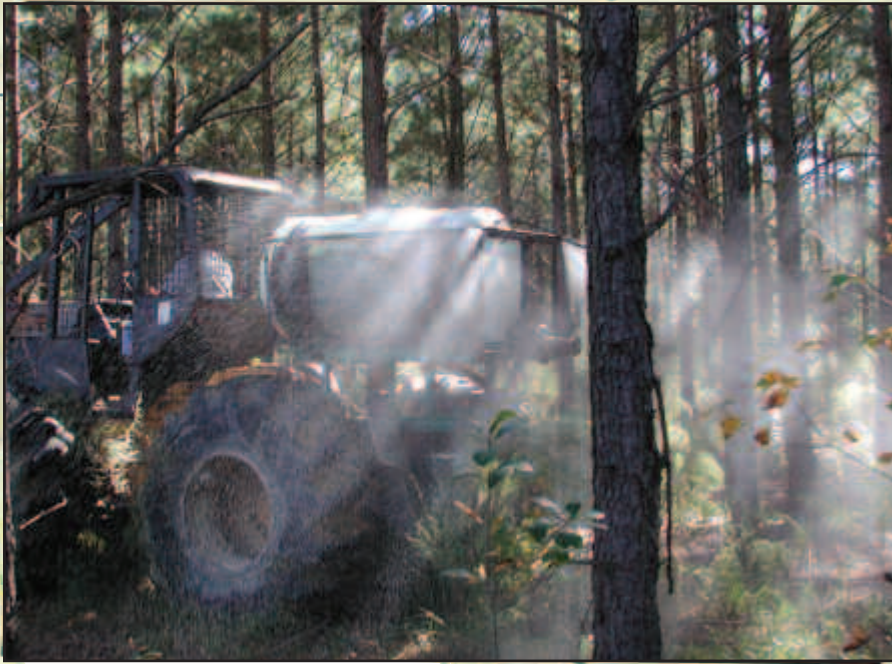
A skidder sprayer applies Arsenal ® to a pine stand.
