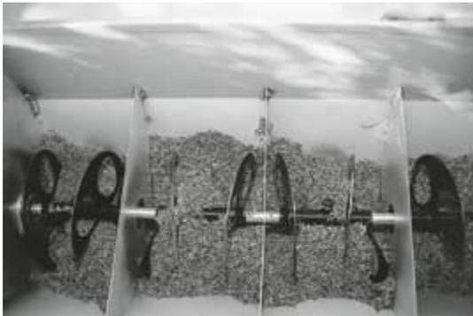
**No-till NWSG drills provide the most consistent results seeding these grasses because they have augers in the hopper and pickers that move seed into the tube.**
